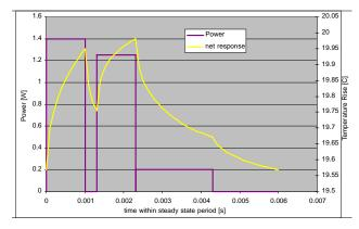
Figure 15. 3–Pulse Periodic Example Steady–State Transient Response
