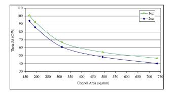
Figure 1. Theta–JA vs. Copper Area for a Dpak
