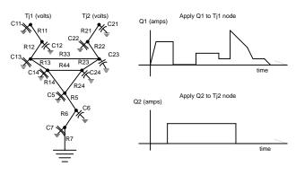
Figure 10. Implementing a Multiple Input Cauer Network in a Circuit Simulator
