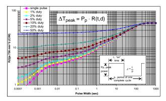
Figure 6. Typical Duty Cycle Curves
