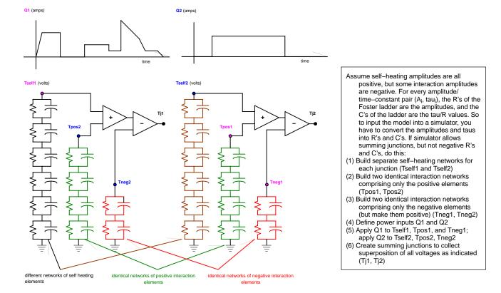
Figure 11. Implementing a Multiple Input Foster Network in a Circuit Simulator
